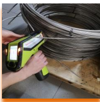
Positive material identification (PMI)
